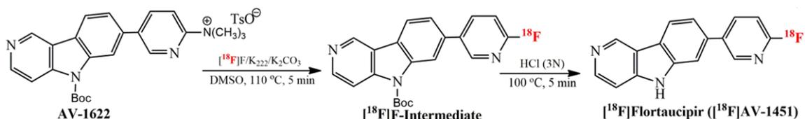
**Figure 1.** Reaction scheme for radiosynthesis of [<sup>18</sup>F]Flortaucipir.
