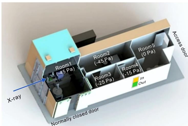
**Figure 1.** Layout of the Biosafety area. Five rooms and corresponding air pressure are shown in the figure.
