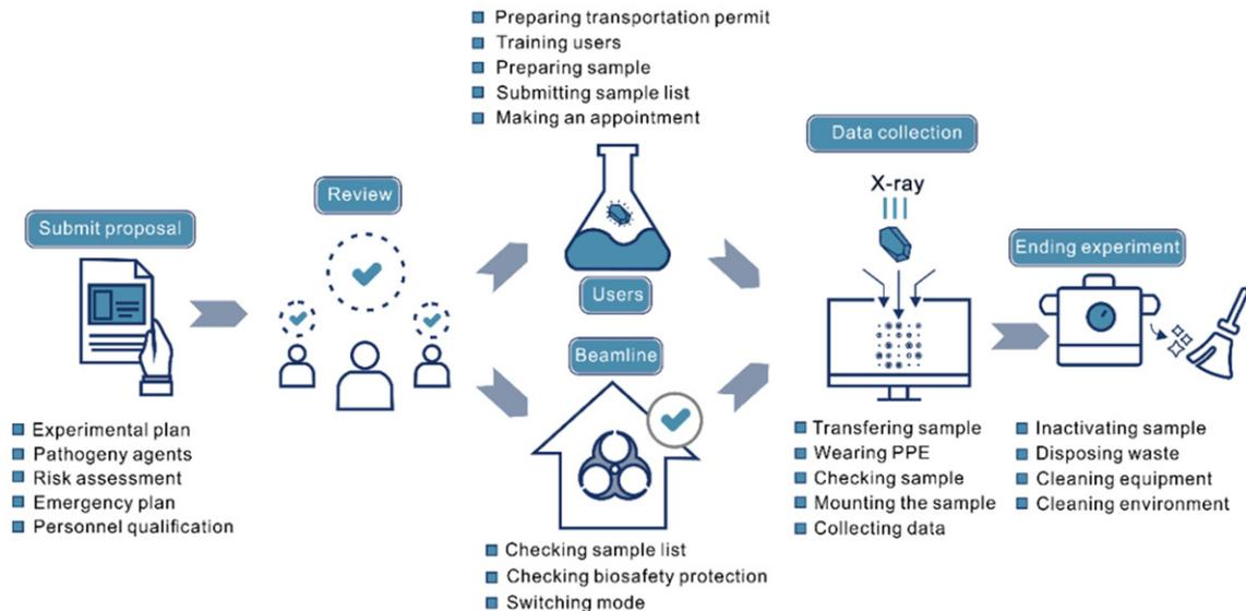
**Figure 3.** Experimental flow chart procedures of proposal submission, review, experimental prepration, in-situ data collection and experiment ending performed in BL10U2.
