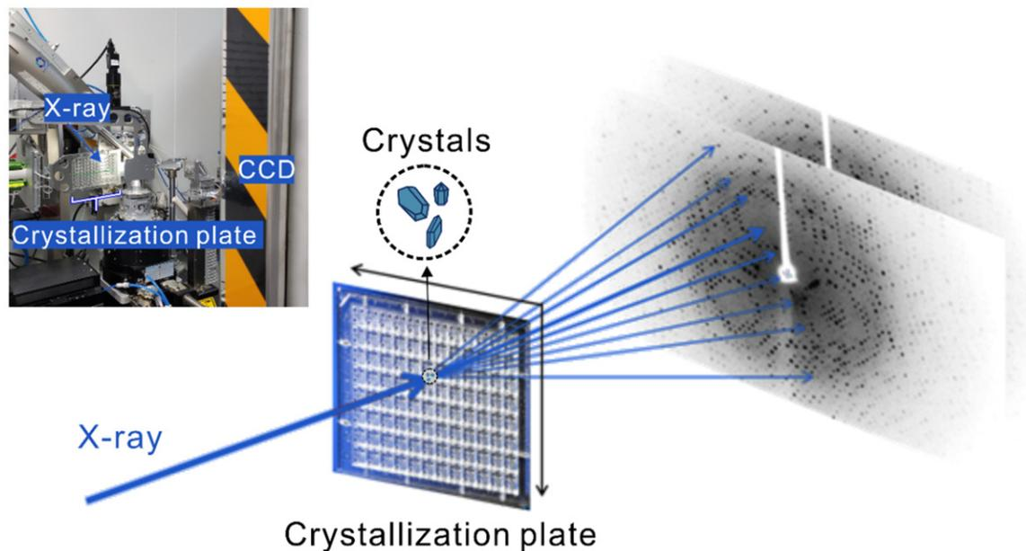
**Figure 4.** In-Situ data collection scheme. The Crystals are sealed in the crystallization plate and moved to the X-ray, and the detector records the diffraction images.
