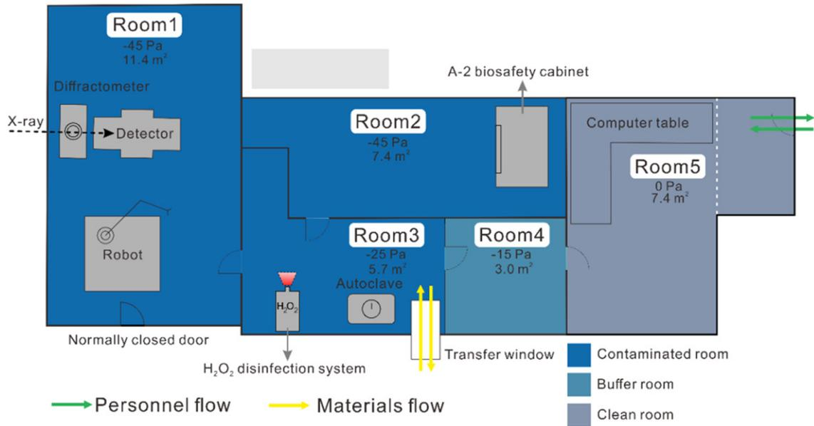
**Figure 2.** Floor plan of the Biosafety area. Major instruments were represented in the figure. The lab is connected to outside through a transfer window. The lab was divided into five rooms, including three contaminated rooms, a buffer rooms and a clean rooms, which are indicated in the corresponding colours. Green lines and yellow lines show the routes for personnel flow and materials flow through the lab, respectively.
