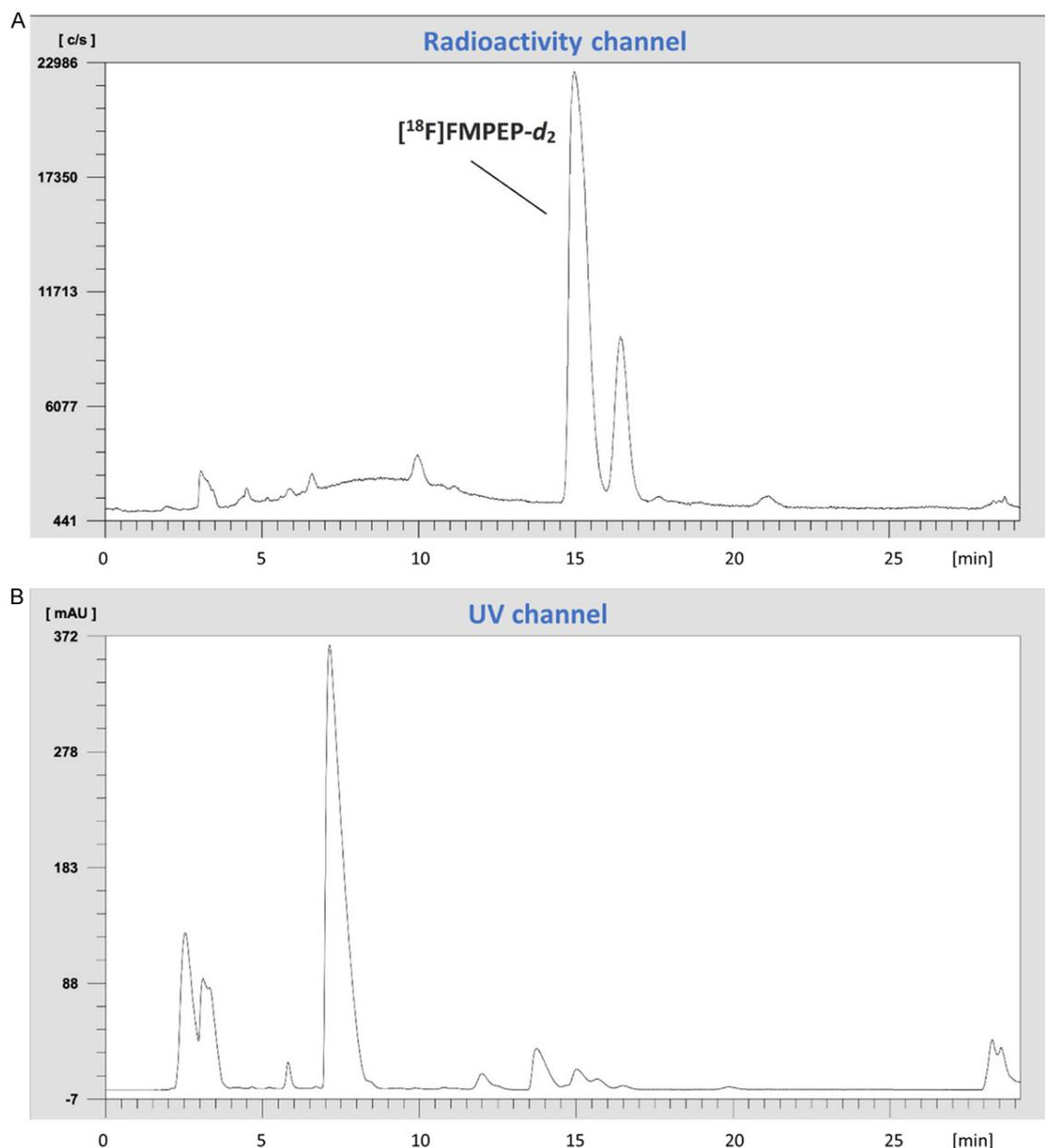
**Figure 4.** Representative semi-preparative HPLC chromatograms for [ $^{18}\text{F}$ ]FMPEP- $d_2$  purification. (A) Radioactivity channel and (B) UV channel.
