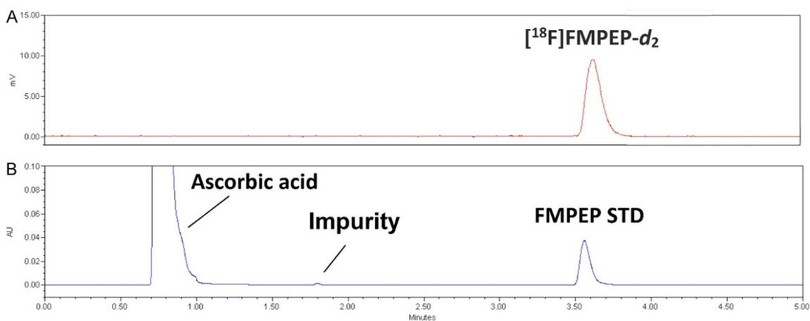
**Figure 5.** Representative analytical HPLC chromatograms of [<sup>18</sup>F]FMPEP-d<sub>2</sub> and reference co-injection. (A) Radioactivity channel and (B) UV channel.
