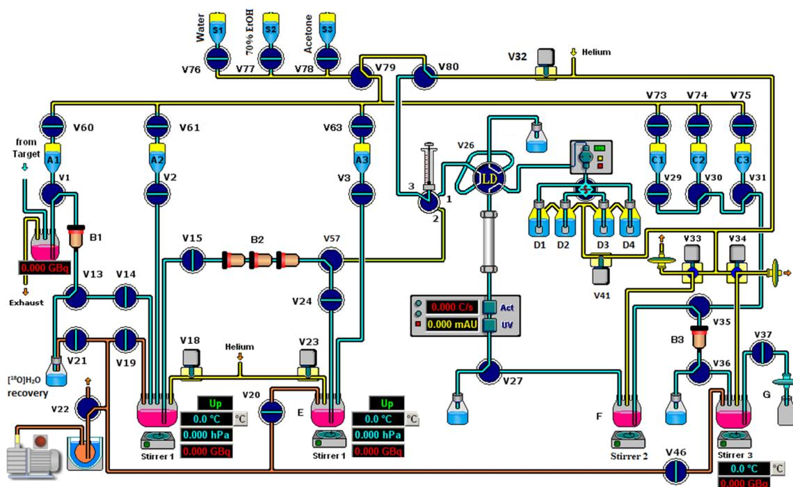
**Figure 3.** Diagram of Synthra RNplus research module for [<sup>18</sup>F]FMPEP-d<sub>2</sub> production.
