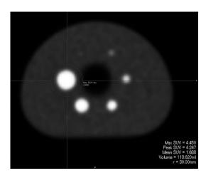
**Figure 1.** A sample PET images of a NEMA phantom with a VOI. Both the SUVmax and SUVpeak of all six spheres (inner diameter 37, 28, 22, 17, 13, and 10 mm) in the phantom were measured using a VOI that covered the whole sphere and was recorded for all reconstructed images.
