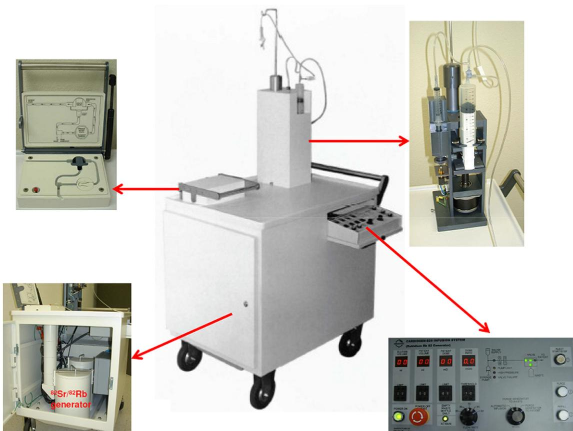
**Figure 7.** Photograph of the CardioGen-82 Infusion System along with various part of the system.
