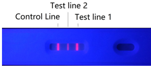
Figure 2. Representative example of the developed test strip. A strip installed in the test card showed a result 15 min after the addition to the card of 75 \mu L sample containing hemoglobin and transferrin. The fluorescent bands were observed under 365 nm ultraviolet light.
