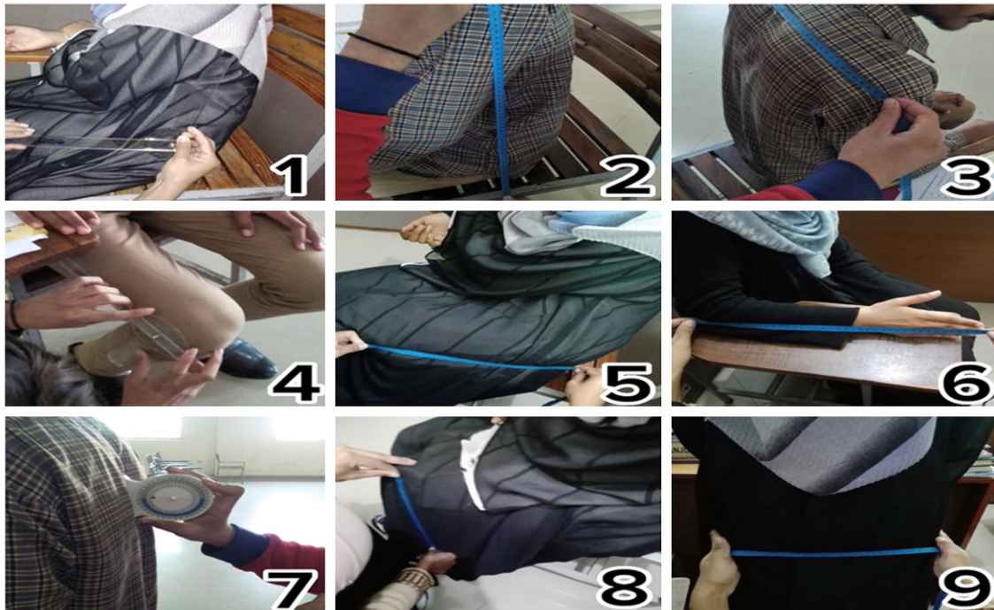
Figure 1. A. Anthropometric dimensions of the students. SHH: shoulder height; EHS: elbow height sitting; SHB: shoulder breadth; PH: popliteal height; KH: knee height; HW: hip width; EFL: elbow-fingertip length; BPL: buttock-popliteal length; ABD: abdominal depth; FW: forearm width; TT: thigh thickness. B. Photographic representation of methodology used for students' anthropometric measurements.
