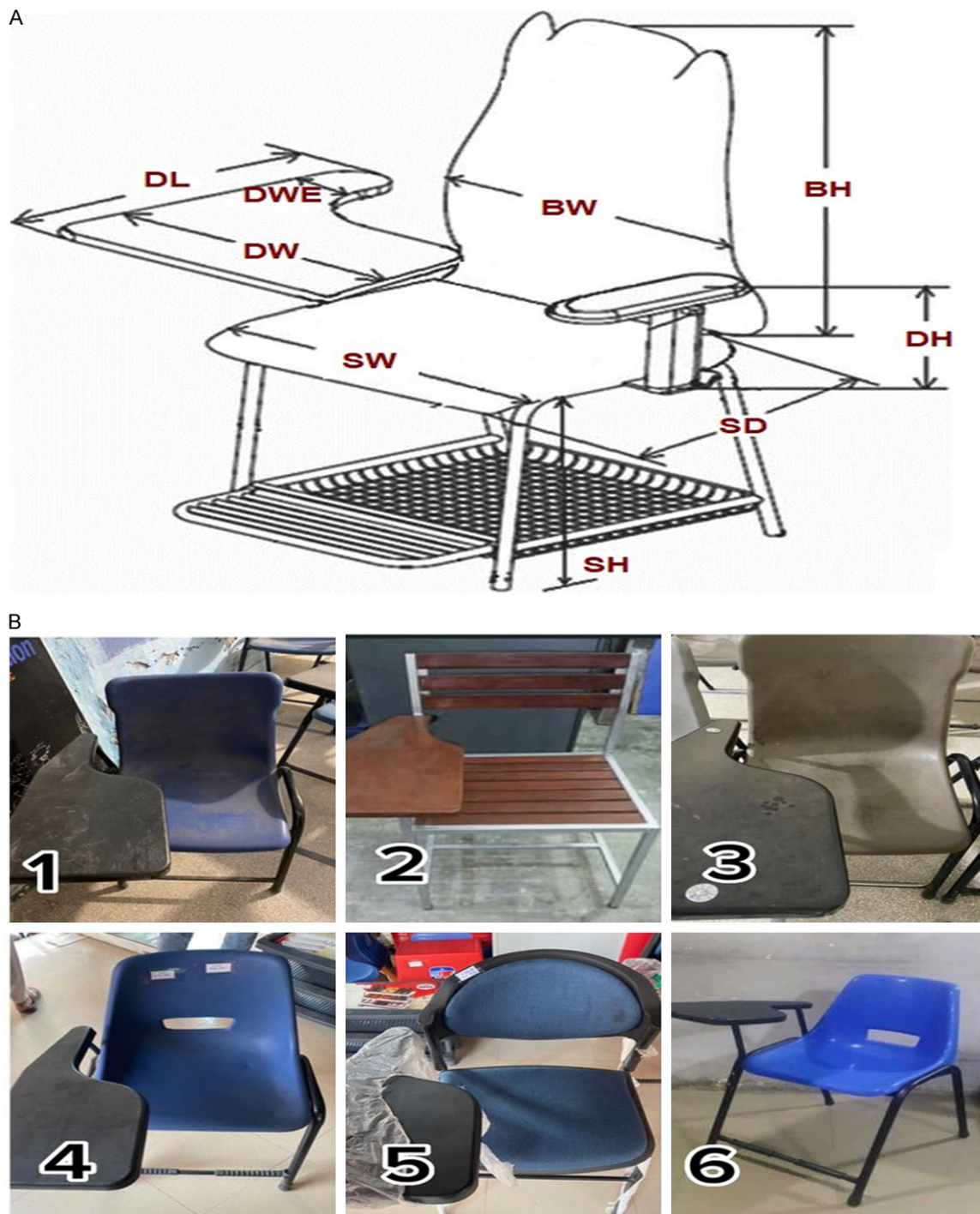
Figure 2. A. Dimensions of the classroom chairs. SH: seat height; SD: seat depth; SW: seat width; DH: desk height; DWE: armrest width elbow; DW: desk width; DL: desk length; BW: backrest width; BH: backrest height. B. Different types of classroom chairs were used in the study.
