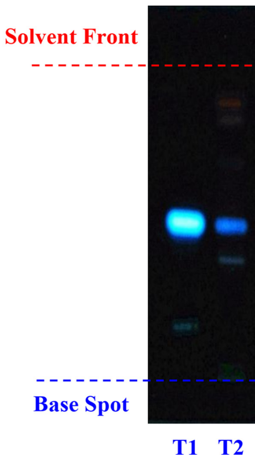
Figure 2. TLC plate of scopoletin standard with EA extract resolving different bands at various Rf values.
