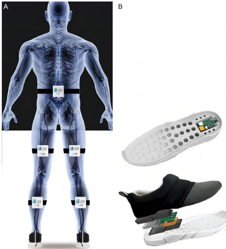
Figure 1. The Gibbon gait analyzer. A: Schematic diagram illustrating the process of gait data collection. B: The device's smart shoe, which is utilized for collecting gait data.
