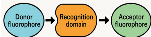
Figure 3. Modular design of the FRET biosensor. FRET: Fluorescence resonance energy transfer.
