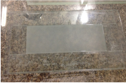
Figure 1. Process for obtaining the porous membrane by solvent evaporation with the addition of sucrose as a leaching agent.
