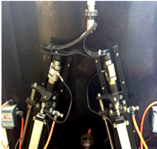
Figure 4. Fatigue property testing machine for prosthetic foot.
