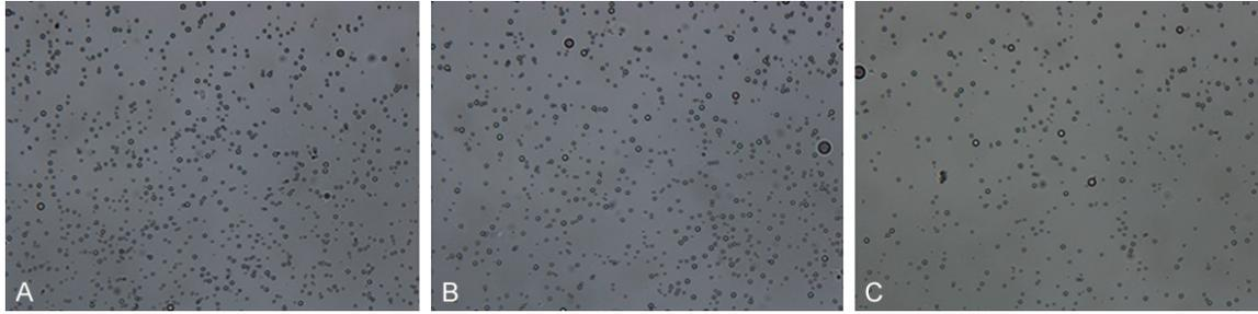
**Figure 1.** A. Optical microscope observation of Targestar SA microbubble contrast agent ( $\times 200$ ); B. Optical microscope observation of Targestar SA microbubble contrast agent + 3 mg of urokinase + 3 mg of RGDS ( $\times 200$ ); C. T Optical microscope observation of Targestar SA microbubble contrast agent + 6 mg of urokinase + 6 mg of RGDS ( $\times 200$ ).
