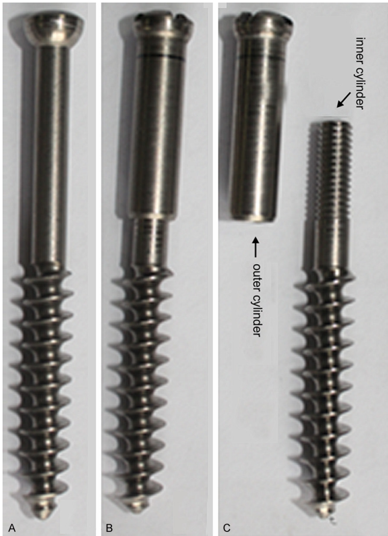
Figure 1. The partially threaded cancellous lag screw (PTLS) and combined partially threaded cancellous lag screw (CPTLS). These screws have identical shank lengths (28.4 mm) and threads (inner diameter: 3.2 mm, outer diameter: 6.5 mm, thread pitch: 2.75 mm, and length: 32 mm). A. PTLS: the shank has a simple structure. B. CPTLS: the shank has a complex structure. C. The CPTLS shank consists of an inner cylinder and outer cylinder. The inner cylinder is contiguous to the thread (outer diameter: 4.5 mm) and contains fine threads on the surface. The outer cylinder is hollow and contiguous to the head (outer diameter: 6.5 mm), and it contains fine threads (thread pitch: 0.85 mm).
