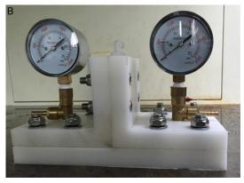
**Figure 1.** A. The map of the T chamber system: the chamber system, 1 reservoir, 2 pump, 3 tube, 4 the T-shape chamber, 5 pressure gauges, 6 flow constrictors; B. The T chamber.
