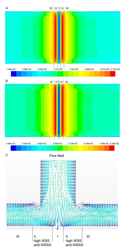
**Figure 2.** A. CFD simulation of WSS and WSSG of the impinging flow in the flow rate of 250 ml/min; B. CFD simulation of WSS and WSSG of the impinging flow in the flow rate of 500 ml/min; C. CFD stimulation for 2D geometry at the rate of 250 ml/min; Three flow zone, velocity magnitude and direction in the T chamber were shown in this image.
