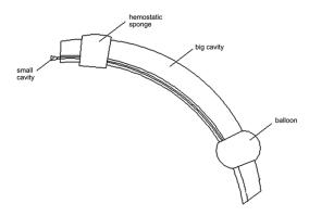
**Figure 1.** Schematic illustrations of thedouble-lumen hemostatic device. The device has two cavities. The large cavity has a function for ventilation and supports the nasal structure, while the small one is used to inflate the air to the balloon.
