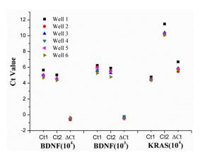
Figure 4. Data distribution of reproducibility assessment on F-CAUM PCR for detecting BDNF and KRAS genes. For detecting the BDNF human genomic DNA standards at  $10^3$  copies/ $\mu$ l and  $10^4$  copies/ $\mu$ l respectively, as well as the KRAS plasmid mixture at  $10^4$  copies/ $\mu$ l six times, the Ct values of Channel 1 and Channel 2 and  $\Delta$ Ct values of Channel 1 and Channel 2 among six replicates showed minimal variance.
