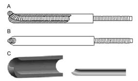
Figure 1. The new multi-directional CD apparatus. This apparatus is constituted by special designed tube within a flexible drill. Frontier of the tube has a side port to going through the drill. Rotate of the tube part plus forward and back the drill part may guide the drill in different direction in core decompression, which would innovatively avoid unnecessary injures. A. Lateral view. B. Aerial view. C. Detailed structure of the tube part.
