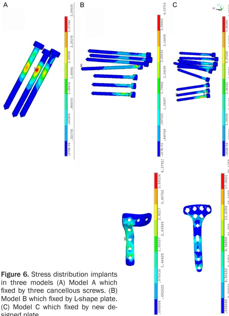
**Figure 6.** Stress distribution implants in three models (A) Model A which fixed by three cancellous screws. (B) Model B which fixed by L-shape plate. (C) Model C which fixed by new designed plate.
