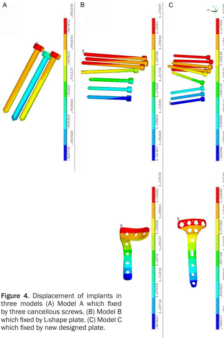
**Figure 4.** Displacement of implants in three models (A) Model A which fixed by three cancellous screws. (B) Model B which fixed by L-shape plate. (C) Model C which fixed by new designed plate.
