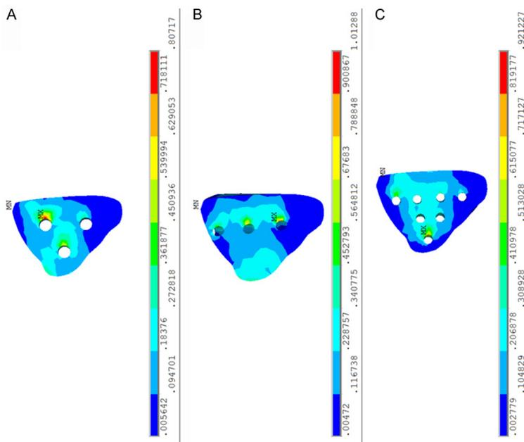
**Figure 7.** Stress distribution of three models on triangular fragment (A) Model A which fixed by three cancellous screws. (B) Model B which fixed by L-shape plate. (C) Model C which fixed by new designed plate.
