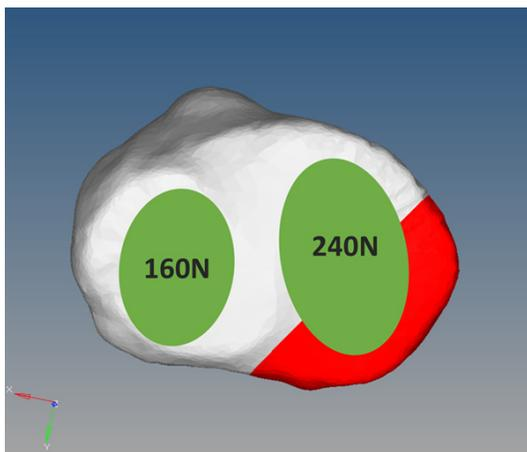
**Figure 2.** Distribution of 400 N axis compression on the tibial plateau articular surface.
