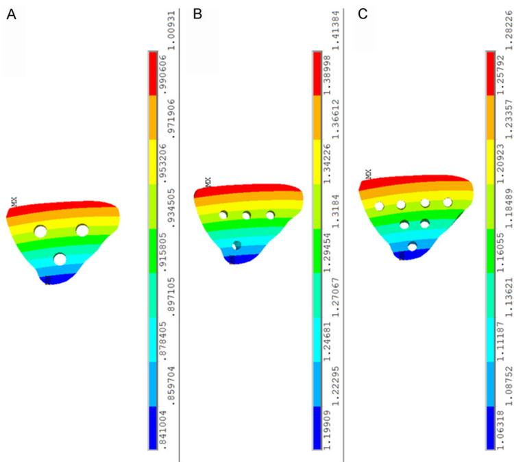
**Figure 5.** Displacement of three groups on triangular fragment (A) Model A which fixed by three cancellous screws. (B) Model B which fixed by L-shape plate. (C) Model C which fixed by new designed plate.
