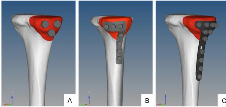
**Figure 1.** Three models after implants assemblage (A) Model A which fixed by three cancellous screws. (B) Model B which fixed by L-shape plate. (C) Model C which fixed by new designed plate.
