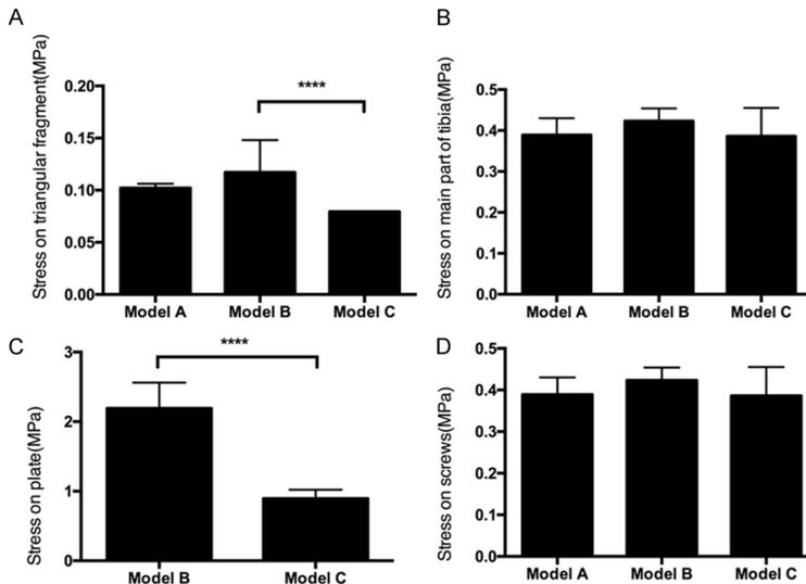
**Figure 9.** Comparison of mean stress value of two models. \*\*\*\* $P < 0.001$ , A. The mean stress on triangular fragment (MPa) after loading. B. Mean stress on main part of tibia (MPa) after loading. C. Mean stress on plate (MPa) after loading. D. Mean stress on screws (MPa) after loading.
