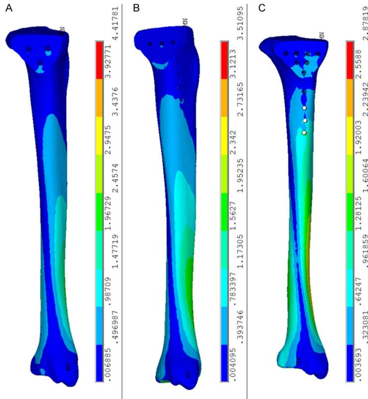
**Figure 8.** Stress distribution of three models on main part of tibia (A) Model A which fixed by three cancellous screws. (B) Model B which fixed by L-shape plate. (C) Model C which fixed by new designed plate.
