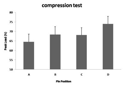
**Figure 4.** Comparison of the peak loads on different pin positions in the compression test. Compared with the other three groups, group A showed basic fixation stability effect at peak load.
