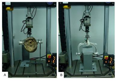
**Figure 3.** Biomechanical test with the base unit of the electromagnetic motion analysis device. A. Skull in the compression test; B. Skull in the tensile test.
