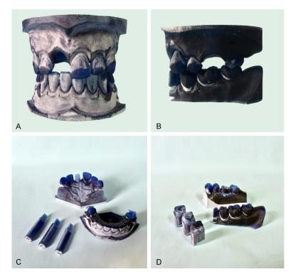
**Figure 2.** A. Models including one vacant site for the prepared central incisor. B. Models including one vacant site for the prepared first molar. C. Prepared central incisors of specific TOC angles inserted into the model for identification. D. Prepared maxillary first molars of specific TOC angles inserted into the model for identification.
