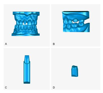
**Figure 1.** A. Standard digital model of maxillary central incisor with neighboring and opposing teeth. B. Standard digital model of maxillary first molar with neighboring and opposing teeth. C. Design of central incisor with TOC of 9 degrees. D. Design of maxillary first molar with TOC of 6 degrees.
