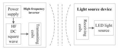
Figure 1. LED light source structure based on wireless transfer power.
