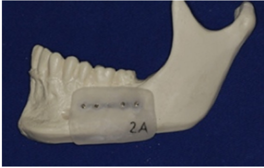
Figure 3. Acrylic model used for the standardized installation of osteosynthesis screws; in this case for group IB.
