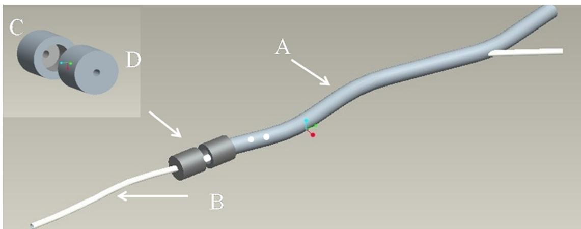
**Figure 1.** The structure of the PB-MA. A: Stent A (bile duct stent), B: Stent B (pancreatic duct stent). C: Magnet C with two central holes (a bigger central hole on one side, a smaller one on the other side). D: Magnet D with a central hole.
