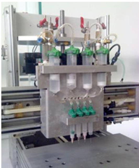
Figure1. 3D cell printer with 4 nozzles for ejecting 4 types of materials/cells.
