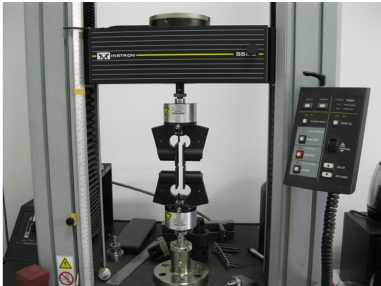
Figure 3. The Instron 5569 material testing machine used to measure mechanical tensile properties of tissue samples.
