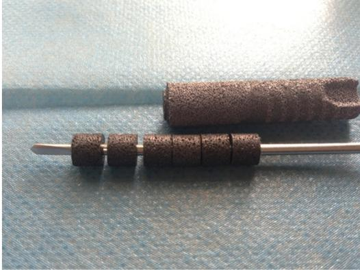
**Figure 1.** Porous tantalum biomaterial specifications. The height was 10 mm, the outer diameter was 8 mm, and a 2.0 Kirschner wire was passed through a central hole with a 2.1 mm diameter hollow area.
