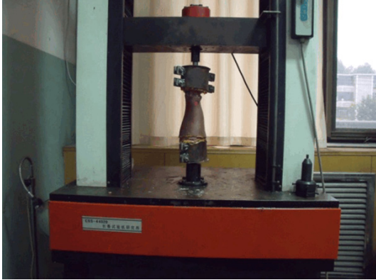
Figure 1. Specimens are mounted on the base of the experimental frame, which was kept in the neutral position.
