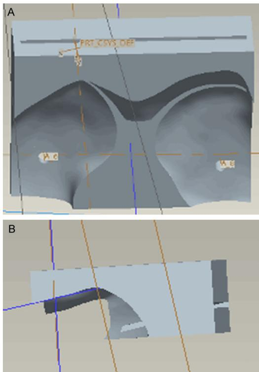
**Figure 4.** Design of the navigational templates. A. Virtual femoral template. B. Virtual tibial template.
