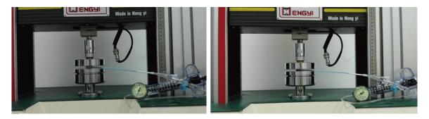
Figure 4. The hydraulic test of Kyphon balloon.
