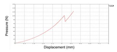
Figure 6. The pressure displacement curve of Kyphon balloon.
