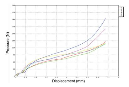
Figure 5. The pressure and displacement curve of EVS biomechanical testing.
