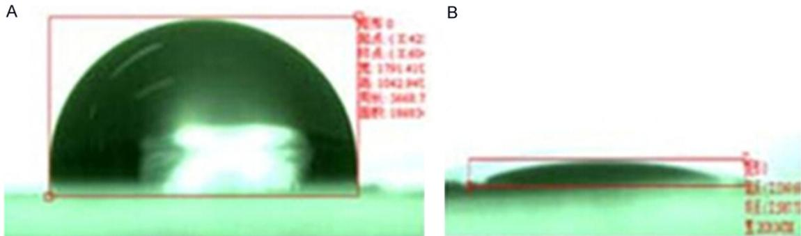
**Figure 3.** Measurement of water contact angle of PHBHHx films. A. Measurement of water contact angle of unmodified PHBHHx films; B. Measurement of water contact angle of PHBHHx modified by PhaP-RGD fusion protein.
