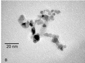
Figure 1. Transmissionelectronmicrograph. A.  $Fe_3O_4$  nanoparticles. B. Polyethyleneimine (PEI)-coated  $Fe_3O_4$  nanoparticles.
