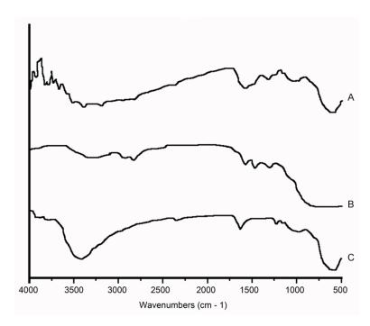
**Figure 2.** Infrared spectrograms for  $\text{Fe}_3\text{O}_4$ , polyethyleneimine (PEI) and PEI-coated  $\text{Fe}_3\text{O}_4$  nanoparticles. A. PEI-coated  $\text{Fe}_3\text{O}_4$  nanoparticles. B. PEI. C.  $\text{Fe}_3\text{O}_4$  particles.
