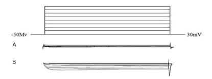
**Figure 1.** Current flow feature of uninduced and induced MSCs. A: No significant channel opening was observed in uninduced and undifferentiated BMSCs; B: Schematic diagram of calcium current after GB-induced differentiation. Calcium currents were detected by applying specified voltages of -50 mV to +30 mV to both groups of cells, where the increment was 10 mV and the duration was 80 ms.
