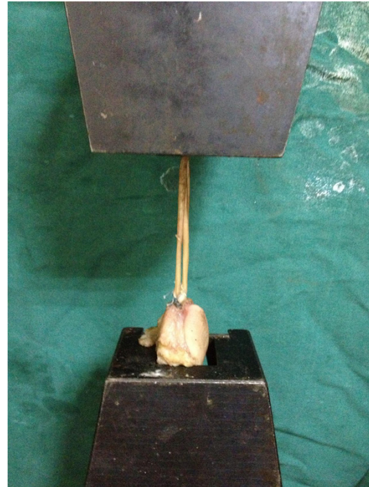
Figure 6. The tendons were fixed to the up side of the testing machine and the patella side was fixed to the bottom of the testing machine.
