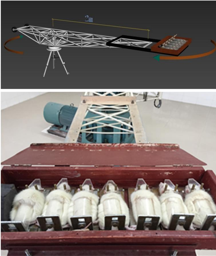
**Figure 1.** The Short-arm Centrifuge for Hypergravity Model. Vertical overload of +10 Gz can be achieved by the animal centrifuge with a diameter of 2 m and programmed by computers. The rats were placed with prone position and head toward the centrifuge axis in the box fixed on the distal end of the centrifuge arm. During the whole centrifugation, the longitudinal axis of the rat body is always parallel to the centrifuge arm.
