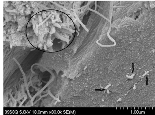
Figure 6. FESEM micrograph where the collagen fibers are surrounded by mineral (circle). Some collagen fibers are trapped within the mineral matrix (arrows).
