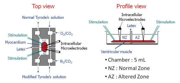
**Figure 1.** Top and profile views of the double compartment tissue bath used for the experiments. The volume chamber of 5 ml enabled the right ventricular strips (slightly longer in rabbits) to be gently passed under the latex membrane in order to have one portion superfused with normal Tyrode's and the adjacent portion with the altered, ischemia-simulating solution.
